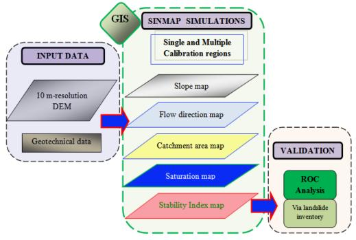
Figure 5 - Generalized methodology flowchart adopting different calibration approaches based on SINMAP (Stability INdex MAPping) model.
