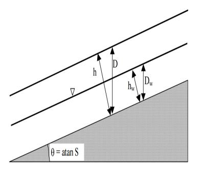
**Figure 3** - Infinite slope stability model schematic. Soil thickness, **h** [m] and vertical soil depth, **D** [m] are related as follows,  $\mathbf{h} = \mathbf{D} \cos \theta$  (Pack et al., 2005).
