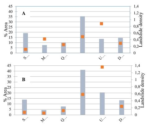
Figure 8 - Prediction accuracy of SINMAP models. A) Model with single calibration region;B) Model with multiple calibration regions (Red squares = landslide density; Light blue bars = area of the stability classes). (S = Stable, M = M = 1Moderately Stable, Q = Quasi-stable, L = Lower Threshold, U = Upper Threshold, D = Defended.
