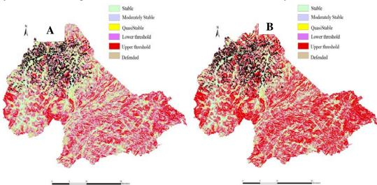
**Figure 10** - Stability Index maps showing the classes of stability obtained by SINMAP calculations in: A) Single calibration region approach; B) Multiple calibration regions approach. (Black dots = location of inventoried landslides).
