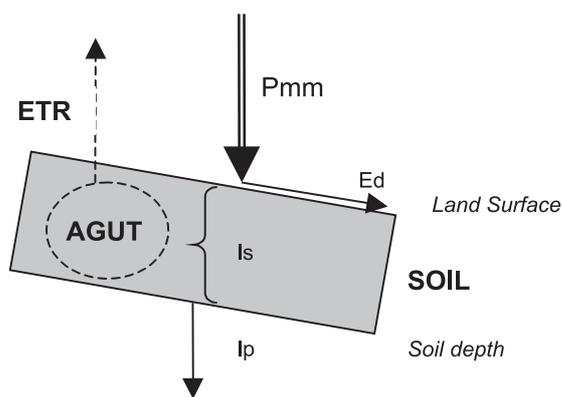
**FIGURE 2.** Soil and topography as factors promoting infiltration (*adapt.* Oliveira et al., 1997).
