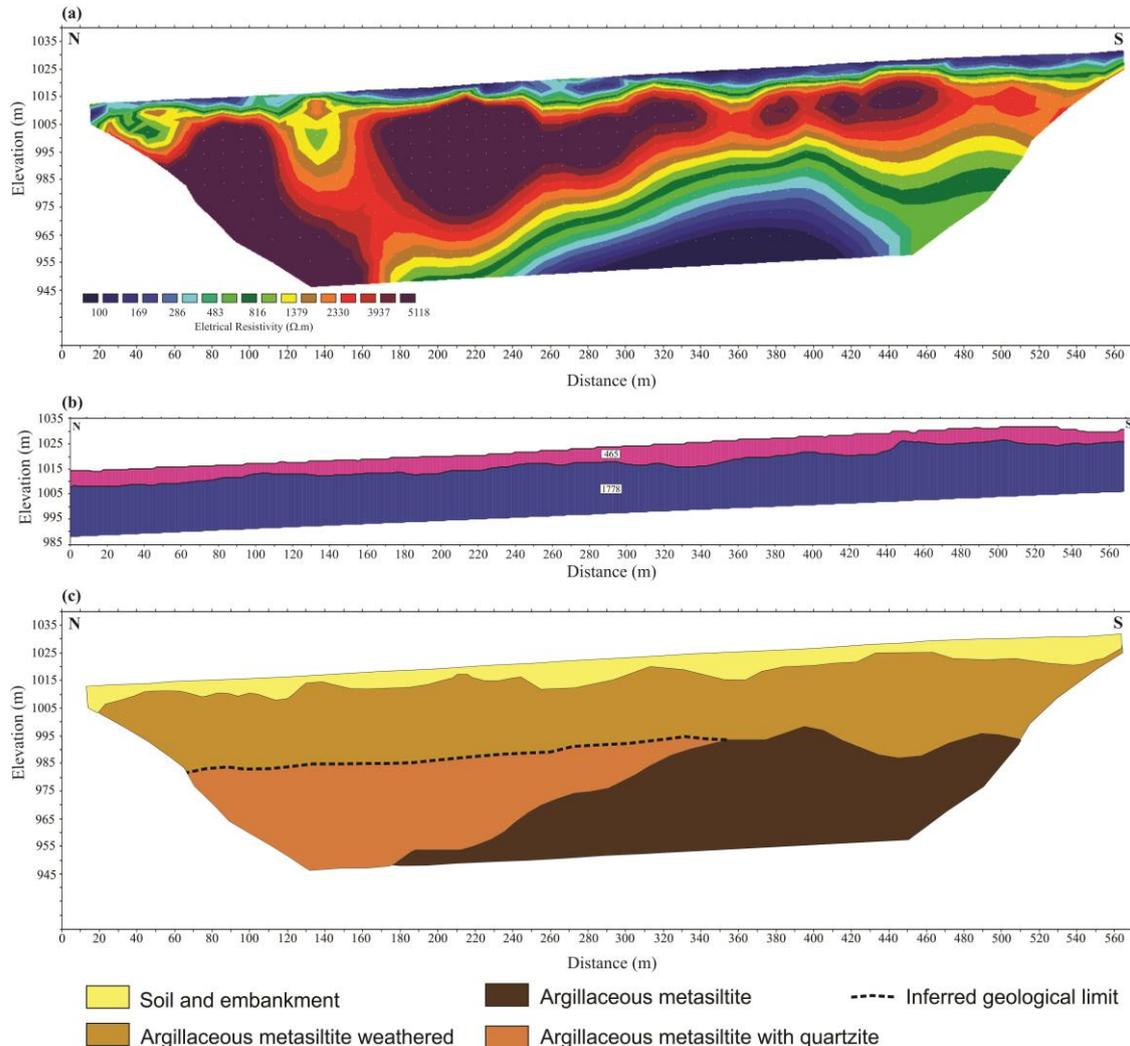
**Figure 4.** Results and model generated. (a) Result of the resistivity. (b) Result of the seismic refraction. (c) Interpretative model.
