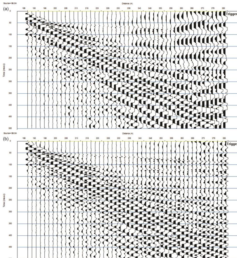
**Figure 3.** (a) Raw data example, showing high level of noise on the farthest geophones. The position of the source point is 186 meters. (b) Filtered data with Low Cut Frequency (LCF) of 37.96Hz.
