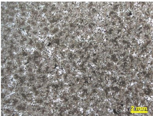
**Figure 2.** Photomicrography of ATP rock showing aphyric and salt-and-pepper texture.
