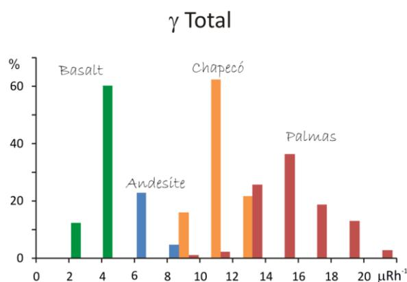
**Figure 14.** Total gamma-ray frequency ( $\mu\text{Rh}^{-1}$ ) histograms for the different volcanic rock types of Serra Geral Formation.
