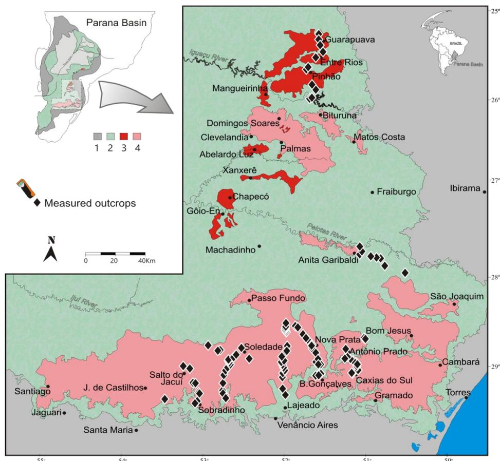
**Figure 1.** Sketched geological map of volcanic rocks of Serra Geral Formation, including gamma-spectrometry measurement location. *Legend:* 1- pre-volcanic rocks, 2- basalts and andesites, 3- Palmas acid volcanics and 4- Chapecó acid volcanics.
