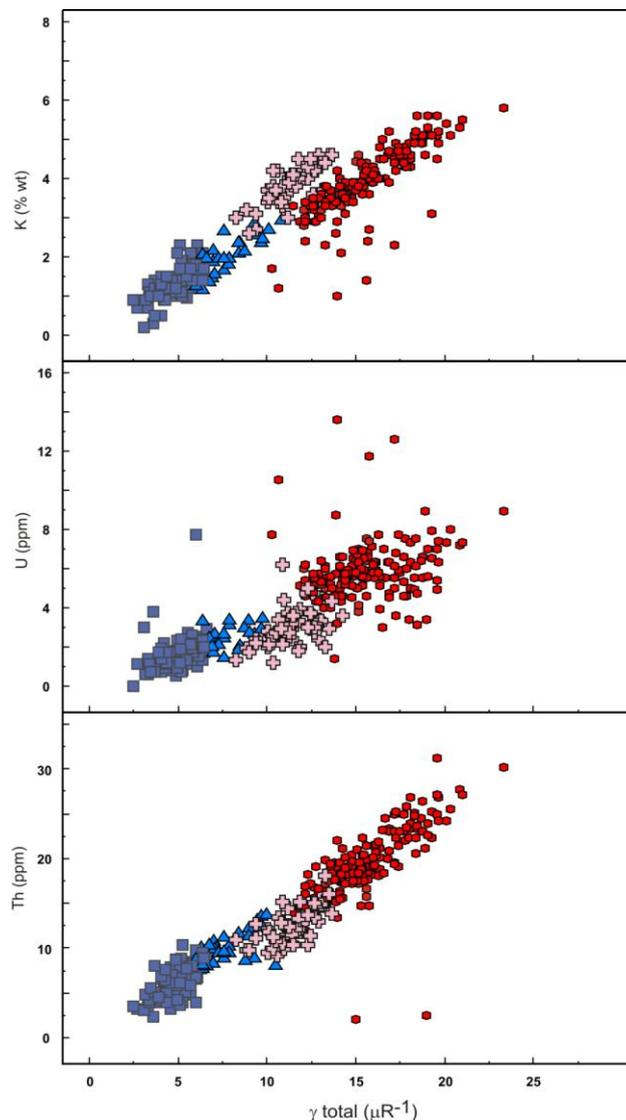
**Figure 15.** Total gamma-ray ( $\gamma$  total) vs K (% wt), U(ppm) and Th (ppm) obtained by gamma gamma-ray spectrometry during the field work. Legend: square= basalts, triangle= andesites, circle= ATP rocks, cross= ATC rocks.
