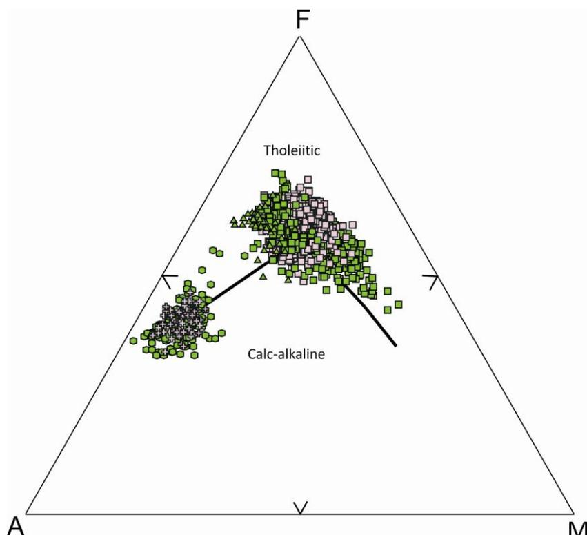
**Figure 12.** A (Na<sub>2</sub>O+K<sub>2</sub>O) – F (FeO<sub>t</sub>) – M (MgO) diagram of volcanic rocks for tholeiitic and tholeiitic-transitional rocks. Legend= as Figure 11.
