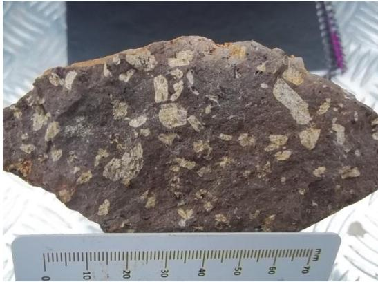
**Figure 7.** Hand sample of ATC rock from Domingos Soraes (PR) showing euhedral plagioclase phenocrysts in a porphyritic texture.
