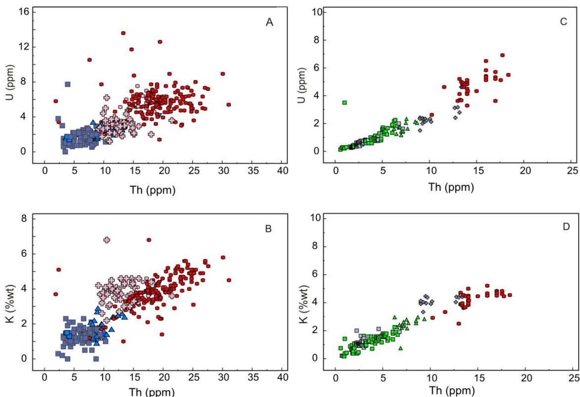
**Figure 16.** Th (ppm) vs. K (% wt), and U (ppm) obtained by gamma-ray spectrometry in this study (A and B) and geochemical data (C and D) from Marques (1988) and Marques et al. (1989). Legend: as Figure 15 (for A and B) and Figure 13 (for C and D).
