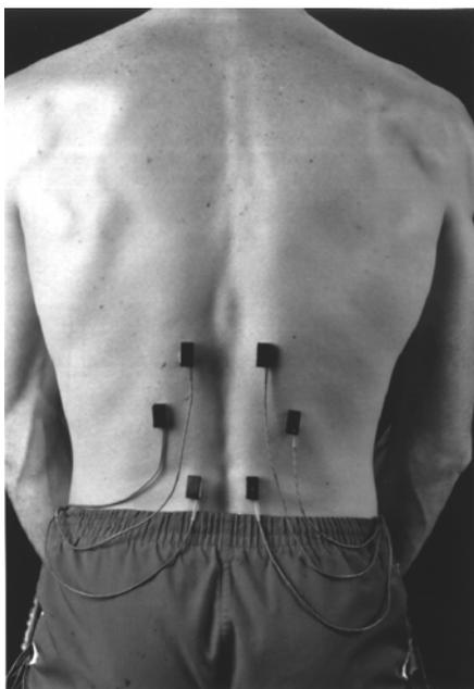
Figure 2. The location of surface EMG electrodes are shown for monitoring changes in EMG spectral parameters during the Back Analysis System test protocol. The muscle sites correspond to Longissimus thoracis, Iliocostalis lumborum, and Multifidus at L1, L2 and L5 spinous process levels, respectively.
